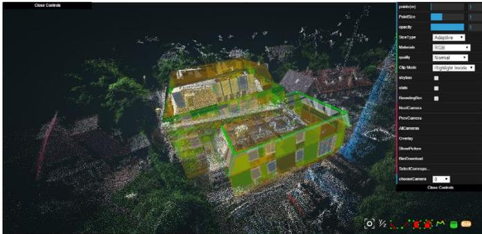
Figure 1 Point cloud comparison with As-Planned .ifc
