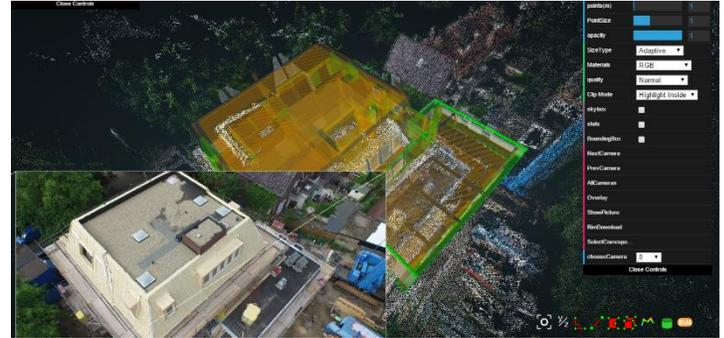
Figure 2 Point cloud comparison with As-Planned .ifc
